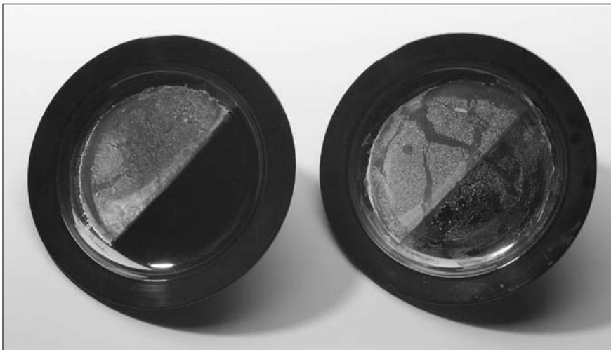
*Dissolving calcium carbonate scale with MGDA (left) and IDS (right)*
